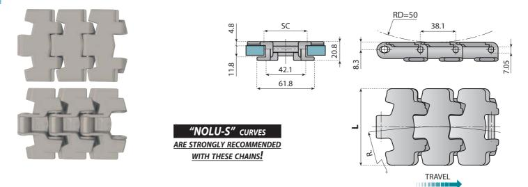
Minimum radius R = 190 mm Recommended curve radius R = 200 mm
